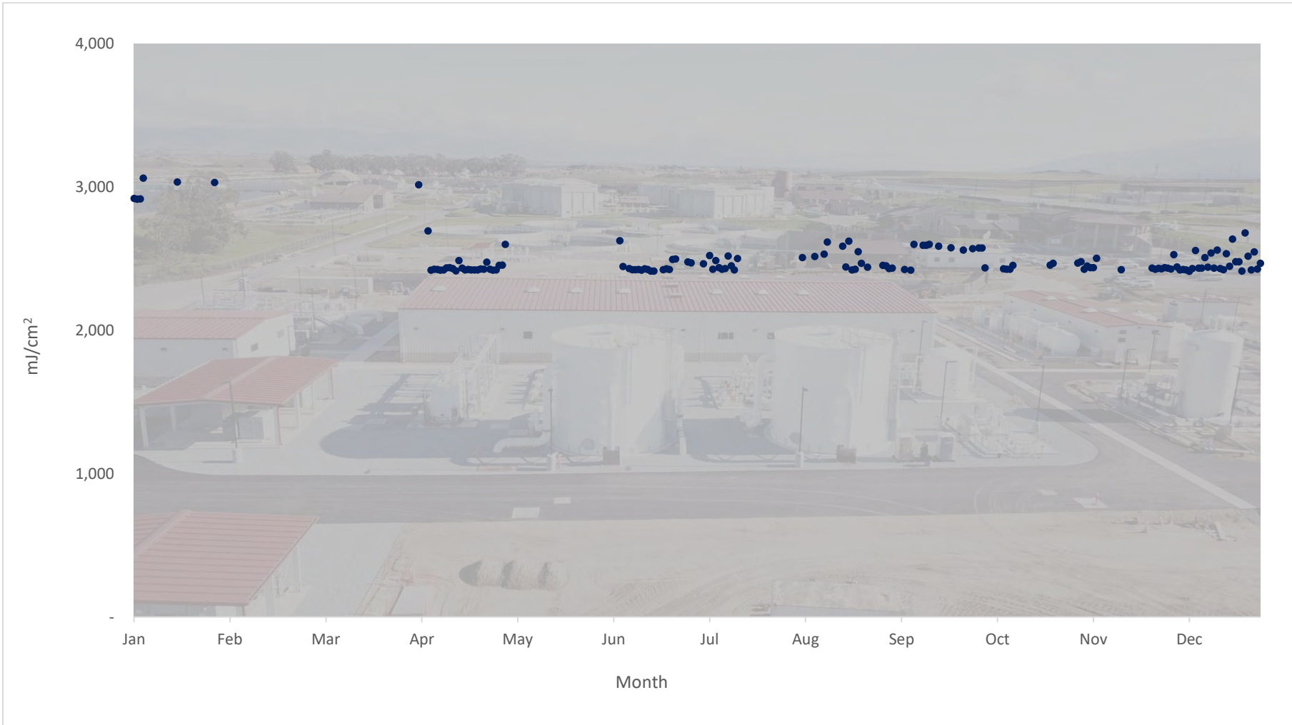
Figure 35. AWPf Product Water Monitoring – Daily Average UV Dose for Reactor 1 (mJ/cm²)
