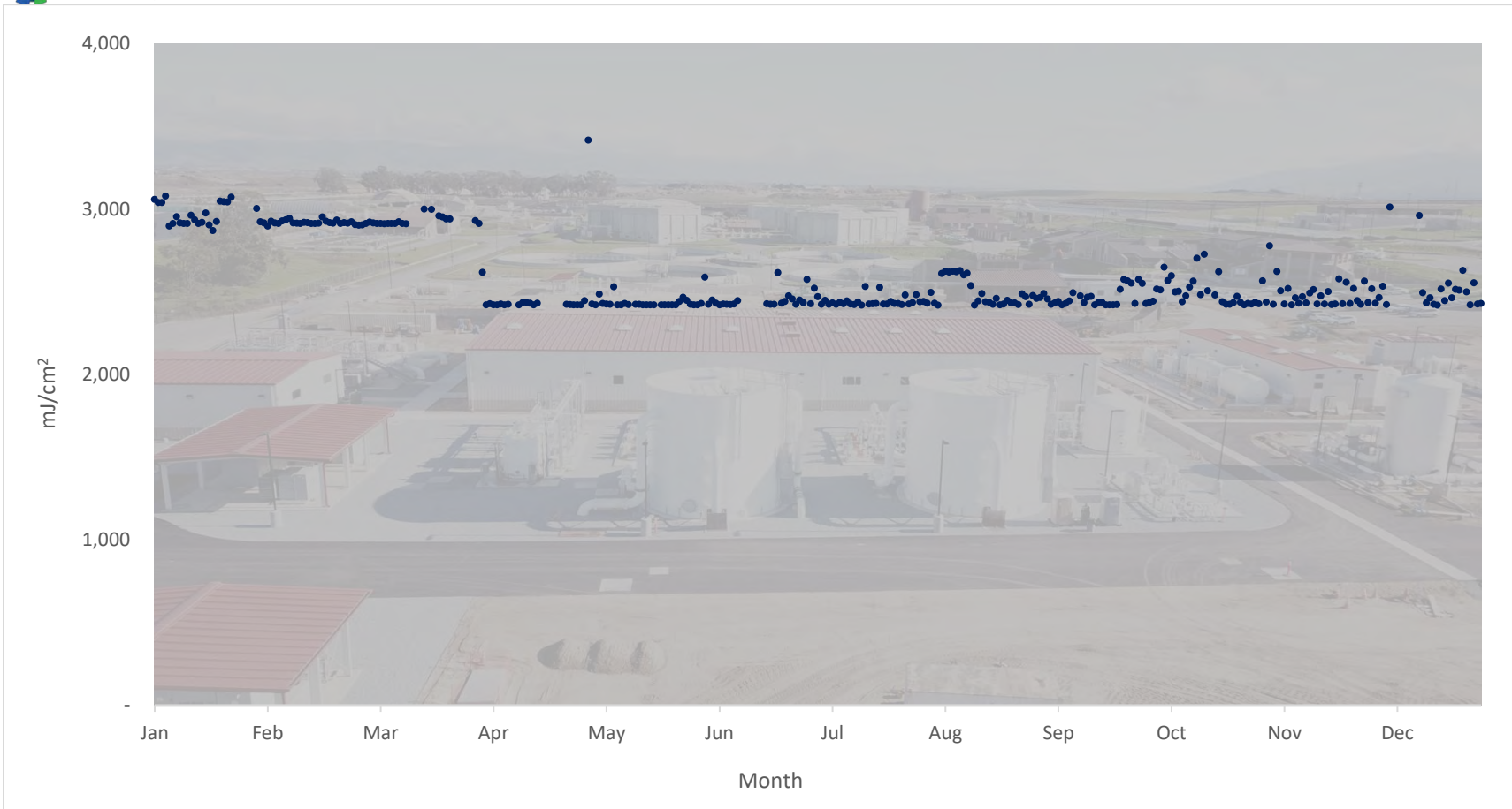
Figure 41. AWPf Product Water Monitoring – Daily Average UV Dose for Reactor 3 (mJ/cm 2 )
