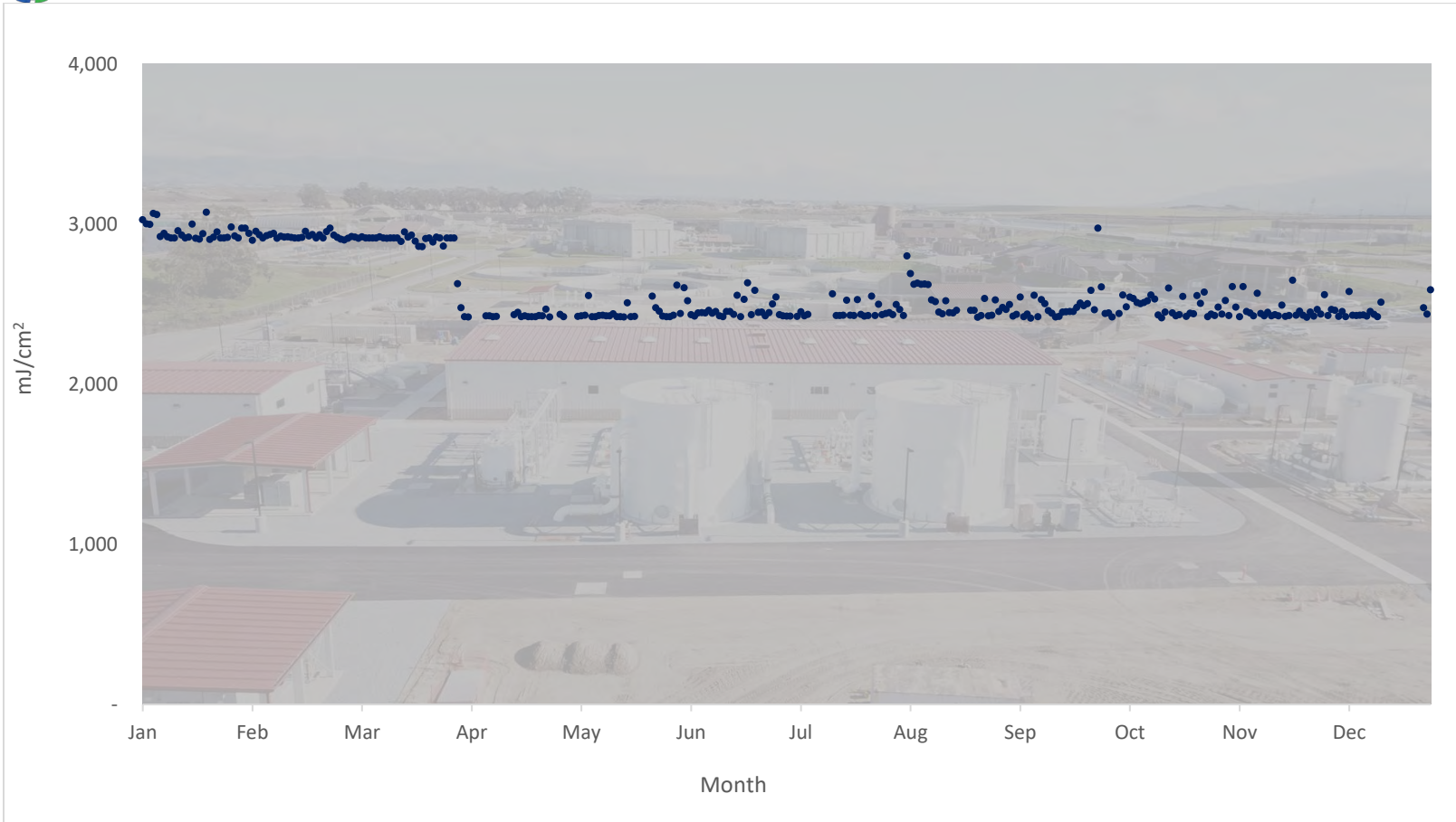
Figure 38. AWPf Product Water Monitoring – Daily Average UV Dose for reactor 2 (mJ/cm 2 )
