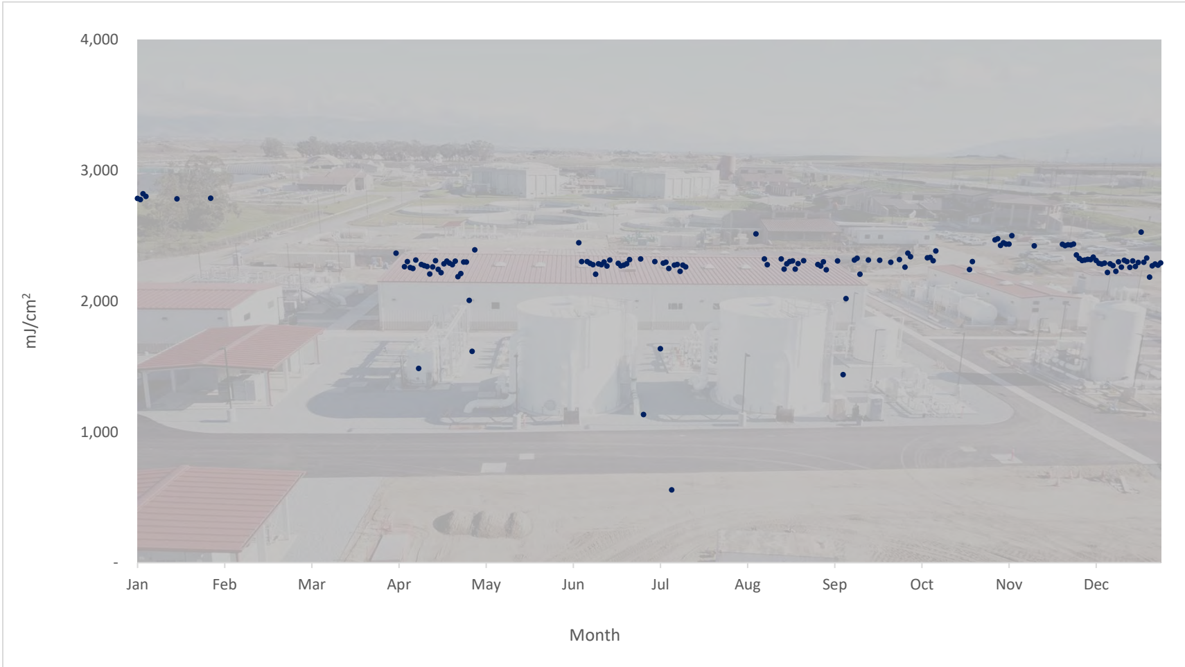
Figure 36. AWPf Product Water Monitoring – Daily Minimum UV Dose for Reactor 1 (mJ/cm 2 )
